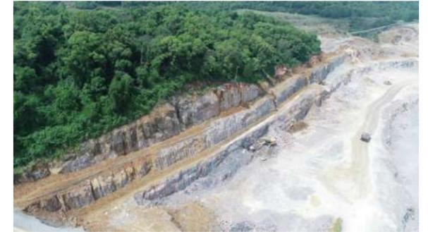
Jiangxi Ya Dong implemented presplit blasting of finished slopes, having maintained the integrity and stability of rock mass
